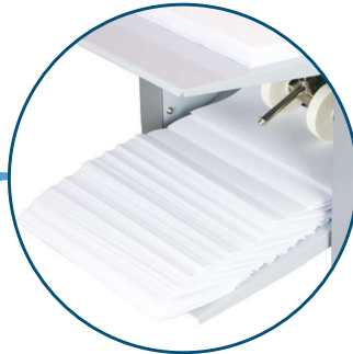
Output Conveyor & Stacker Wheels Stacker wheels can be adjusted for neat and sequential stacking
