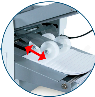
AutoStack™ Stacker Wheels Fully automated to adjust for various form sizes
