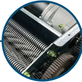
Commercial Grade Heat-treated solid steel cutting blades, all metal gears, AC geared motor
